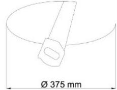
Luminaire must not be covered with insulating matting.
